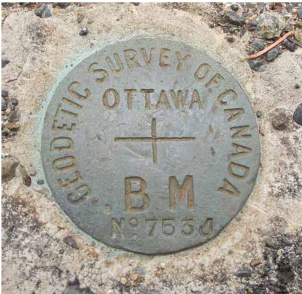
Figure A6–4. A geodetic survey benchmark.
