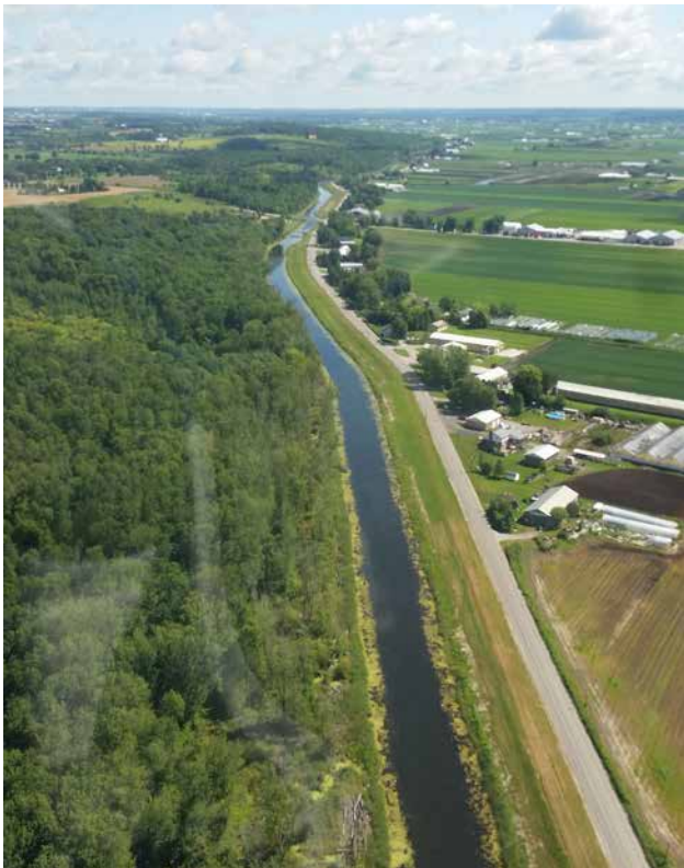
Figure B10-28. An aerial view of a dyke constructed along the full length of farmland that it is protecting from flooding.
